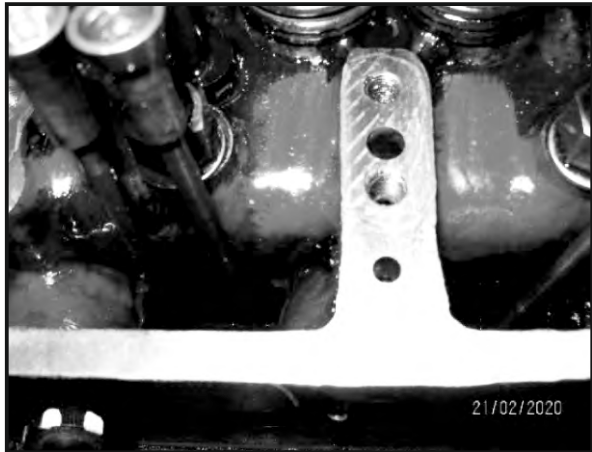
B254FS Modified rear rocker pillar - prevents oil from leaking into coolant owing to porous casting in head - supplied with full instructions
