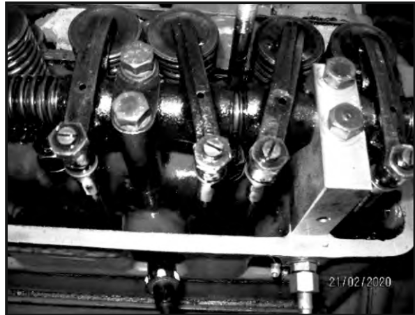
B254FS Modified rear rocker pillar - prevents oil from leaking into coolant owing to porous casting in head - supplied with full instructions
